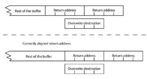
In order to properly align the section of repeated return addresses, an additional 2 bytes should be added to the NOP sled:
