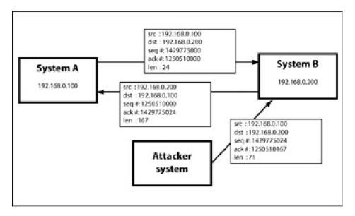
The attacker has forced the victim's connection with the host machine into a desynchronized state. And because the attacker sent out the first spoofed packet that caused all this chaos, the attacker can keep track of sequence numbers and continue spoofing packets from the victim's IP address to the host machine. This lets the attacker continue communicating with the host machine while the victim's connection hangs.
