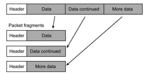
The packet is broken up into smaller packet fragments that can pass through the network link, IP headers are put on each fragment, and they're sent off. Each fragment has a different fragment offset value, which is stored in the header. When the destination receives these fragments, the offset values are used to reassemble the IP packet.
