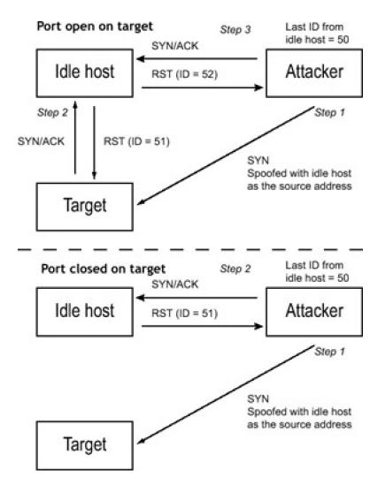
Of course, if the idle host isn't truly idle, the results will be skewed. If there is light traffic on the idle host, multiple packets can be sent for each port. If 20 packets are sent, then a change of 20 incremental steps should be seen for an open port, and none for a closed port. Even if there is light traffic, such as one or two non–scan-related packets on the idle host, this difference is large enough that it can still be detected.
