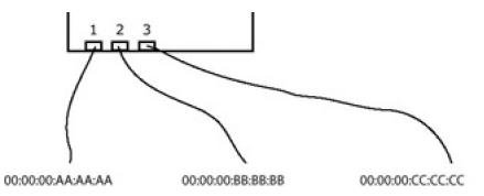
The advantage of a switched environment is that devices are only sent packets that are meant for them, meaning that promiscuous devices aren't able to sniff any additional packets. But even in a switched environment, there are clever ways to sniff other devices' packets; they just tend to be a bit more complex. In order to find hacks like these, the details of the protocols must be examined and then combined.
