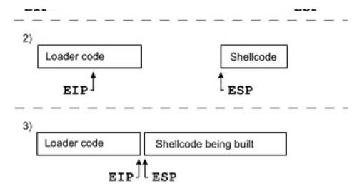
Because the stack grows up (from higher memory addresses to lower memory addresses), the ESP will move backward as values are pushed to the stack, and the EIP will move forward as the loader code executes. Eventually EIP and ESP will meet up, and the EIP will continue executing into the freshly built shellcode.
