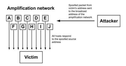
This amplification of traffic allows the attacker to send a relatively small stream of ICMP echo request packets out, while the victim gets swamped with up to a couple hundred times as many ICMP echo reply packets. This attack can be done with both ICMP packets and UDP echo packets. These techniques are known as *smurf* and *fraggle* attacks, respectively.
