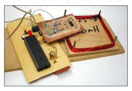
I built the reader on two printed circuit boards. The largest one contains a PIC16F877, used to generate the 125 kHz square wave, and the circuit to drive and tune the coil. The reader coil is a  $\sim$ 1.6 mH inductor wound from about 140 turns of 30 gauge magnet wire on a 2.5" square form.
