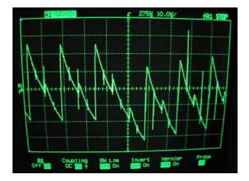
A bit time is 256  $\mu$ s. The tag's id is periodic over 64 bit times, 16384  $\mu$ s. When there is no phase shift, the signal is a 125 kHz sinusoid slightly modulated by a 62.5 kHz sinusoid. The modulation is greatly exaggerated in the figure.
