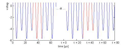
Since a bit time is 256  $\mu$ s, phase shifts are an integer multiple of 256  $\mu$ s apart. Thus, in the above picture, we could have t = 256, 512, 768, ...  $\mu$ s.
