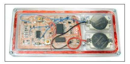
I left the wires long so that I can remove the board from the plastics without desoldering anything. This is necessary to put it on the programming jig, and it helps when I'm trying to figure out whether I have a circuit-does-the-wrong-thing problem or a 125-kHz-pickup-on-everything problem.
