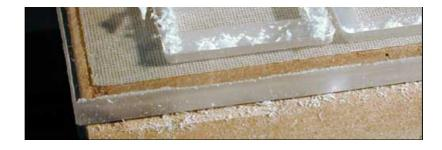
The top and bottom of the case are each 1/16" Lexan (polycarbonate); the core is milled from 6 mm Lexan sheet. The top has drilled holes for the actuators of the two tact switches on the PCB. I paid too much (more than a dollar each!) for the battery holders shown below because they make it very difficult to apply a reverse voltage to the circuit by mis-inserting the cell. The pink foam presses the board into contact with the lid so that the tact switch actuators project.
