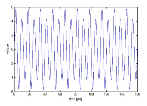
To indicate a bit transition, the tag inserts a phase shift of  $\pi$ . There is always an even number of carrier cycles between phase shifts, so that if the most recent phase shift was achieved by skipping a small-amplitude cycle then the next phase shift will be achieved by skipping a large-amplitude cycle.
