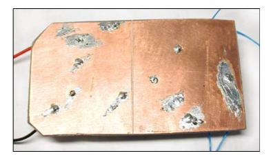
There are no connectors on the board because I couldn't find any low-profile surface mount connectors that I liked. Instead there are test points to program the PIC and tune the coil; I actually built a test/programming fixture (with pogo pins). This is pretty easy with a CNC machine. Power and coil leads are soldered directly to the board. The blue wires are mostly test points, for debugging only. The 8 pin header connects to my PIC programmer.
