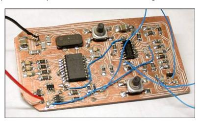
For a sense of scale, the PIC16F628 (largest IC) and the opamp are both SOICs. There aren't any unreasonably fine-pitch components on this board; the tightest are the SuperSOT FETs (bottom left), with 0.95 mm lead spacing.
