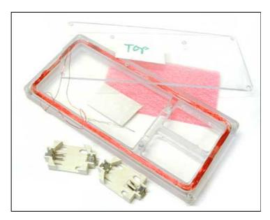
Both the top and bottom screw into the core with #2 tapping screws. I put a lot of effort into finding a local source for a methylene chloride solvent cement (so that I could weld the bottom on instead of screwing it) but I gave up after many failures. I first tried machine screws but small-diameter machine screws tend to have too many threads per inch to work in plastics. Next time I'd probably look for threaded inserts.
