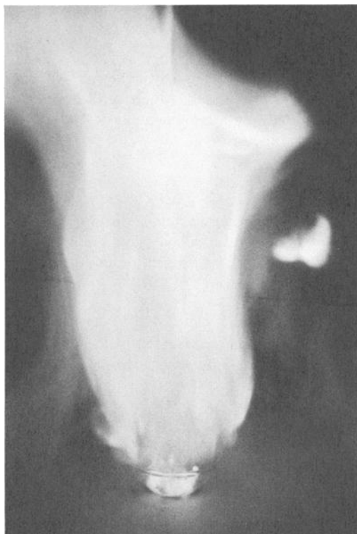
FIG. 1—Fireball produced by the reaction between swimming pool chlorine and brake fluid.
