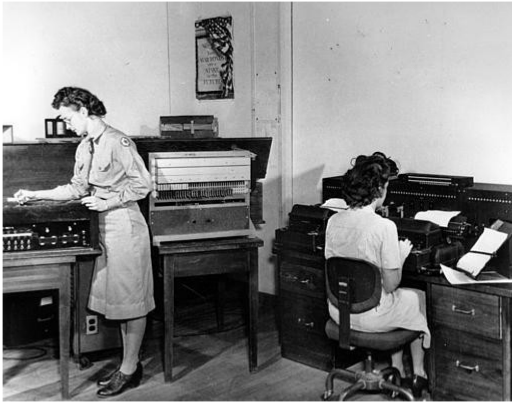
Two intelligence analysts work at two Purple code machine analogues at the headquarters of the U.S. Army cryptanalysis service in Arlington, Va. in 1944 during World War II. The analogue machines, devised by American cryptographers, enable Purple-coded Japanese messages to be deciphered. (AP Photo)
