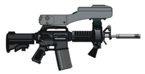
Figure B-14. Rifle-Mounted HIDRAH.
