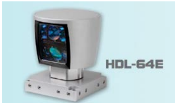
Figure 2. Velodyne Scanning Laser (from www.velodyne.com )
