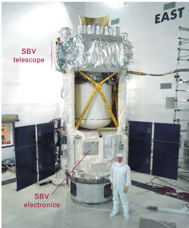
FIGURE 1. The Midcourse Space Experiment (MSX) satellite undergoing final integration and test at the Vandenberg Air Force Base launch processing facilities. The Space-Based Visible (SBV) sensor is composed of a telescope assembly, shown at the top of the satellite, and the electronics assembly, shown near the bottom of the satellite.
